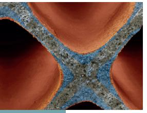
THREE-WAY CONVERSION CATALYST REDUCES EXHAUST GAS EMISSIONS
