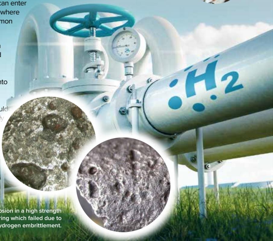
Figure 2: Corrosion in a high strength steel RV spring which failed due to hydrogen embrittlement.
